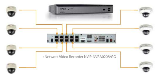
Dome cameras NVIP-2DN2001D/IR-2P/GO
