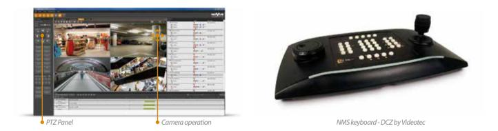
NMS software supports keyboard with joystick, connected to a workstation through the USB port. The keyboard controls a camera and allows to perform basic functions of NMS (ex. switching of views, playback).
